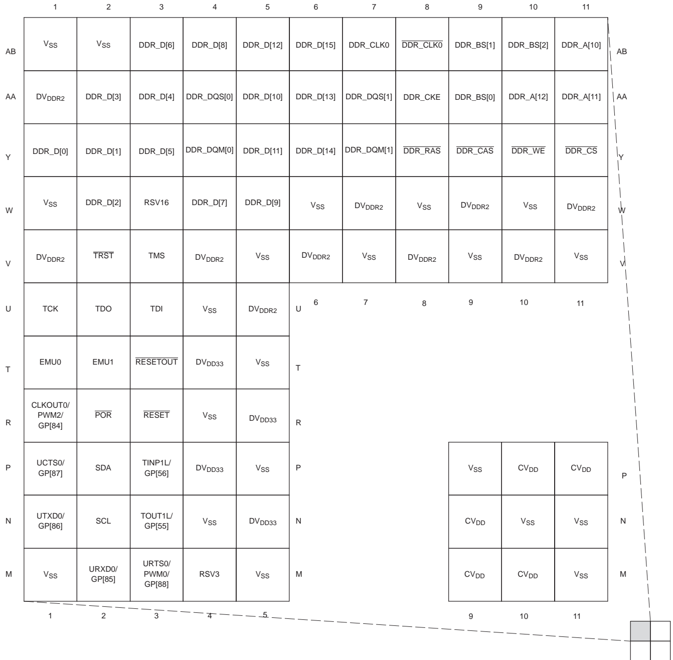
Figure 2-8. ZDU Pin Map [Quadrant A]
